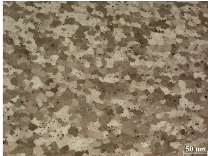
Figure 4. The stirred zone image inside the welded joint is in the middle position of the welded joint.
